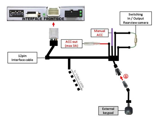
1 Connect the keypad's female 4pin connector to the video-interface's male 4pin connector.
