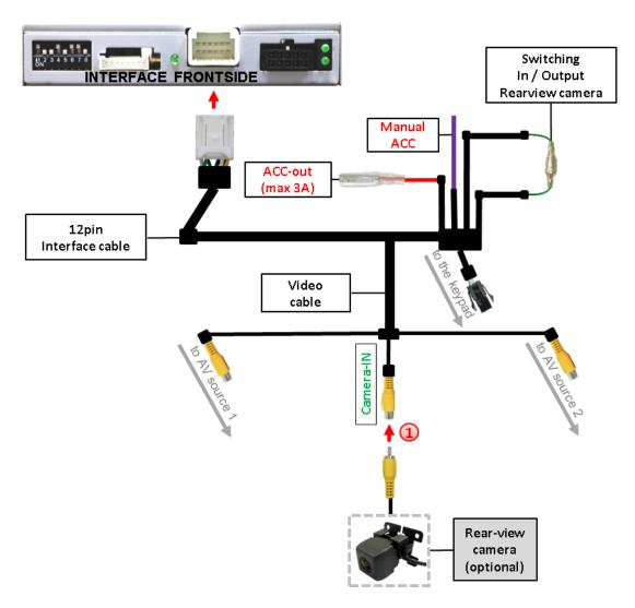
1 Connect the video-RCA of the after-market rear-view camera to the female RCA port "Camera-IN" of the video-cable.
