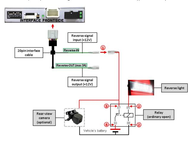
Disconnect the green cable's pre-connected male- and female connectors of the 20pin cable and connect the green input cable "Reverse-IN" to the output connector (87) of the relay.
