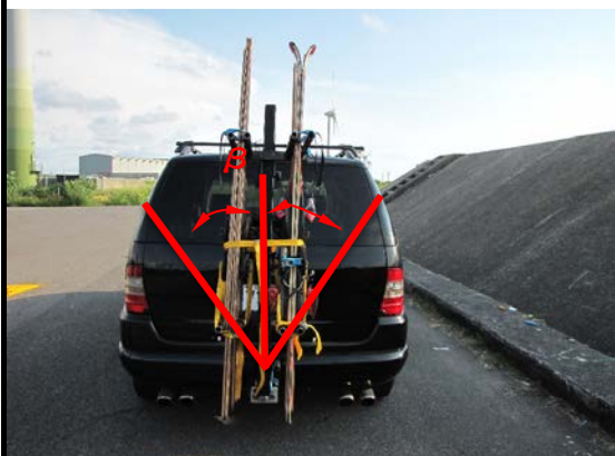
Figure 3 - Application of the angle measure on the test bicycles
